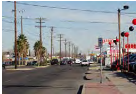
In some areas sidewalks are better maintained and not directly adjacent to travel lanes. However, frequent curb cuts create many conflict points creating less safe and uncomfortable conditions for those walking or on two wheels.
