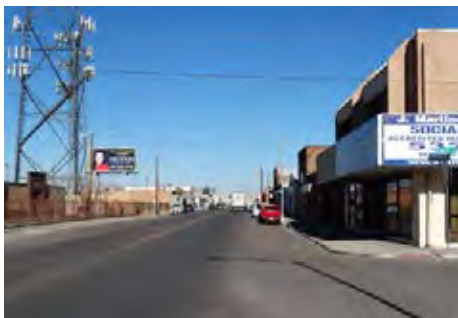
Texas Avenue has a wide curb to curb dimension that includes two wide travel lanes and on-street parking. There is an opportunity to repurpose some of the pavement to better support new development with wider sidewalks and street trees.
