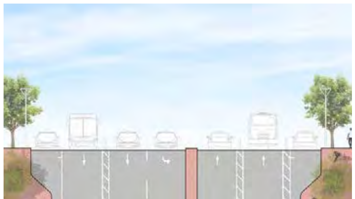
Short-term dedicated bus lane along Alameda Avenue, where space is maintained for other curbside uses, such as parking, loading, or bulb-outs.
