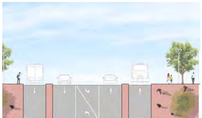
The long-term design for a dedicated transit lane along Alameda includes wider sidewalks and concrete curbs to physically separate the bus lane from vehicular traffic.
