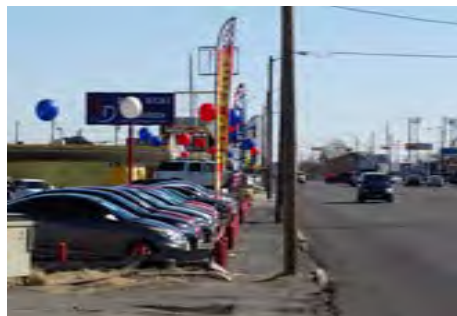
Narrow sidewalks and sidewalks in poor condition are common, with only six inches of curb separating those on the sidewalk from speeding cars.
