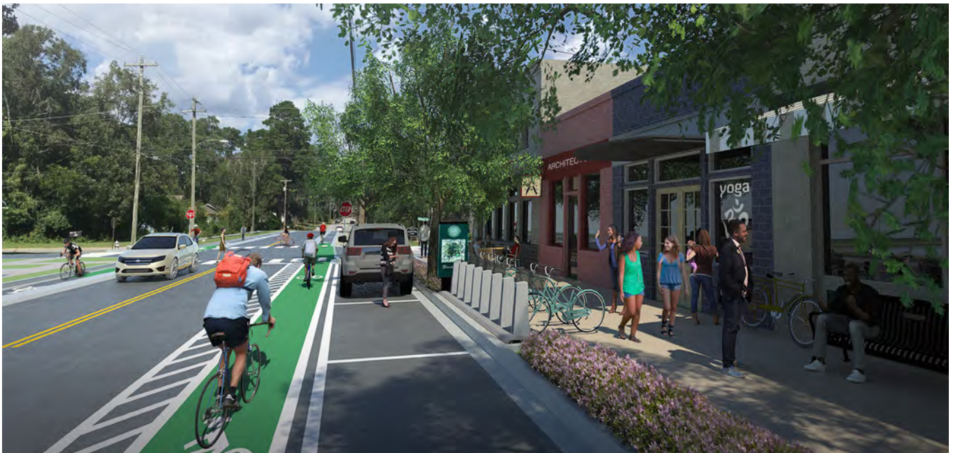
Parallel parking and bike lanes help reduce the travel lanes, increasing pedestrian safety, and promote an active lifestyle.
